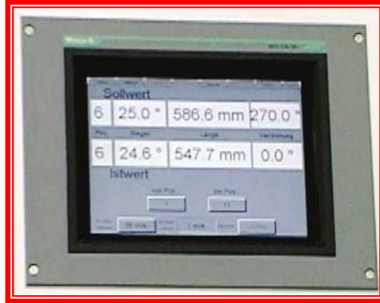
SPS control panel
