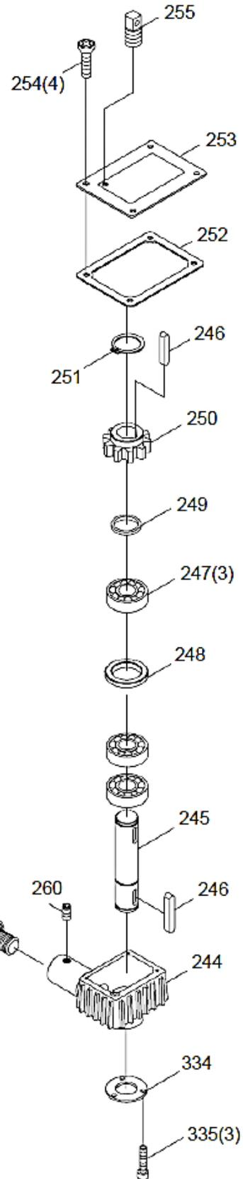
**A3\*: Worm Gear Shaft Assembly**
