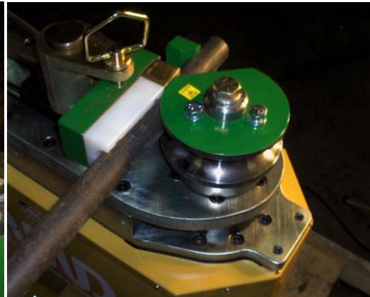
Figure 5 inserting material to start bending
