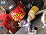
Using a TIG welder, Gary Simpson of Outcast Kustoms in Eagan, MN, tack welded a series of indexed sections in the same primary all held together by the easy to use tack welding clamps.
