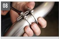
The icengineworks<sup>™</sup> tack welding clamps are an absolute pleasure to work with. The clamps create strong temporary joints, which ensure a gapless welding surface and allow hands-free tack welding of complex sections. We can't help but wonder why they weren't invented sooner.
