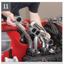
With the header completely tack welded, including the collector, we test fit it in the vehicle to verify the plastic model hadn't shifted or changed in any way from the initial design. Even a slight change could've led to fitment issues with the steel version.
