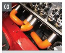
The icengineworks<sup>™</sup> Pro Kit includes eight block adapters, which anchor the blocks in starter tubes. The adapters expand when tightened and prevent the initial block in the header primary from rotating. We designed our header from the top down, starting after the two-inch starter tubes.
