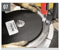
To cut a section out of a six-inch CLR mandrel bent tube, we installed the pivoting table on our vertical band saw along with the corresponding six-inch CLR spacer and started cutting. The table and spacers ensure precise cuts that are always perpendicular to the centerline, which greatly simplifies the welding process.
