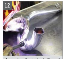
Once we knew the steel header fit as well as our icengineworks  $^{\text{\tiny TM}}$  3D model, we gave Gary the green light to begin the finish welding. Notice the D-shaped end of the tube; Gary formed the tube to fit the header flange perfectly, which matches the exhaust ports in the cylinder head.
