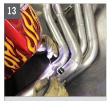
Gary used silicon bronze filler rod for both the collector and the flange welds to ensure quality penetration and a strong seal. The clean and precise welds produced by a TIG welder are second to none. From our experience, TIG welding is the only way to go when building custom headers.
