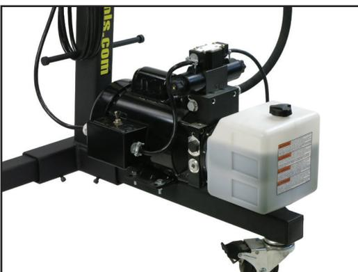
10. - Attach pump as shown in the photo using the included 5/16" hardware.
