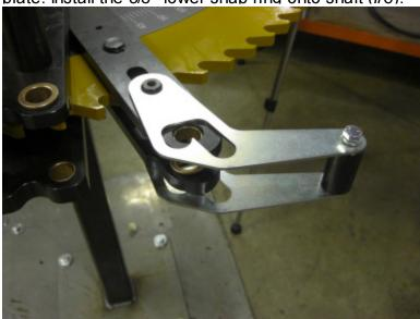
29) Install pivot pin (#12) through drive link, lock tab slots, upper drive bar, the drive link again, lower drive bar, and finally the lower lock tab. Install snap rings on both sides, as shown below.
