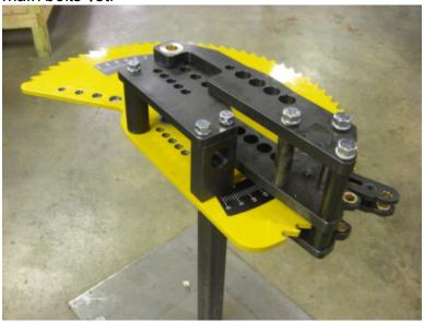
25)Now that the majority of the machine is built, the drive lever section can now be assembled, use Dwg #M050-EV3. Locate the 2 drive links (#2) and the shaft block (#4). Bolt together using (8) 5/16-18 X 1" as shown below.
