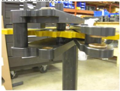
27) Install snap ring onto shaft (#11) and slip through drive link end hole through middle and bottom plates, and install lower snap ring to shaft (#11) as shown below.
