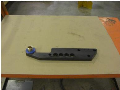
21) Install the hook drive plate. This must be oriented correctly as it can be put on backwards, see picture below.
