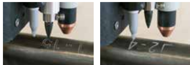
Tube marking/etching: Bend-Tech Dragon obtains the bending information from the Bend-Tech Industrial software to automatically mark and etch bend angle labels, bend locations and rotations.
