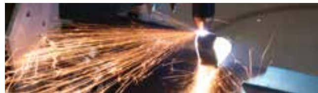
Plasma cutting: Cuts end profiles, holes, and other contours.
