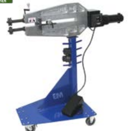
24" Deluxe kit shown with industrial motor. Includes 5/16" round bead, 1/16" step, and spoiler rolls, rolling stand, roll holder, and depth stop
