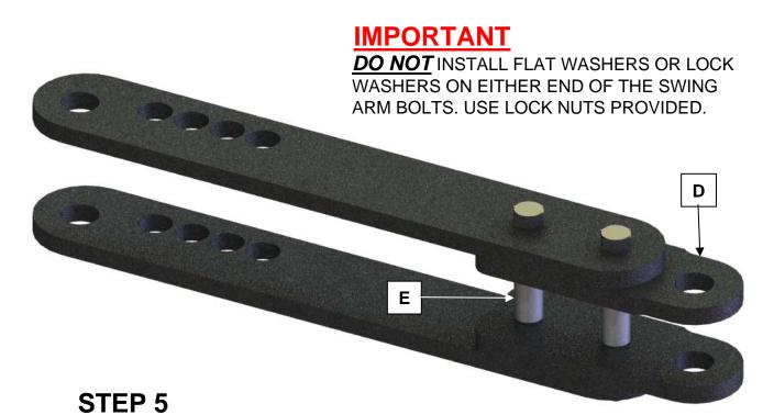
RE-ASSEMBLE SWING ARM AS SHOWN ABOVE, USING EXTENSION PLATES (D) AND SPACERS (E) PROVIDED. ATTACH SWING ARM TO BENDER.
