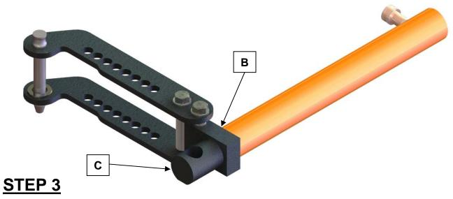
B) SCREW HYDRAULIC CYLINDER AS FAR AS POSSIBLE INTO THREADED HOLE OF YOKE.
