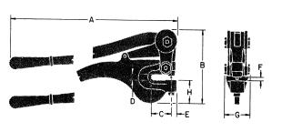
**CARE:** Oil at hinge points, punch guide hole in Frame (1), and Punch (14) point.
