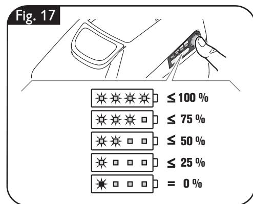
The real percentage of the battery charge condition is only indicated when the power tool motor is stopped.
