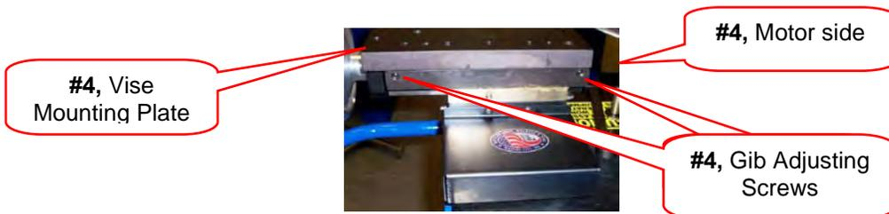
5. Once you are satisfied with the adjustments tighten the five gib mounting bolts and recheck your adjustments. This procedure may take a few tries. You can now remount the vise to the mounting plate.
