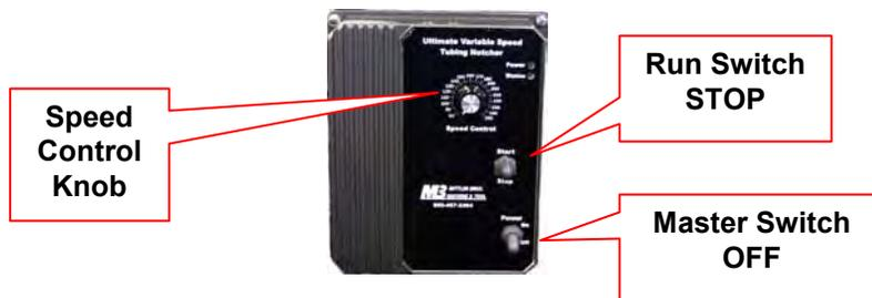
19. Turn the **MASTER** switch on and then turn the **RUN** switch on. Turn the speed control knob up and down to cycle the motor. Listen for and clicking or odd sounds. If you hear a clicking sound you will need to loosen the spindle housing bolts and then retighten while the motor is running. This will usually align the Love Joy and quiet the clicking.
