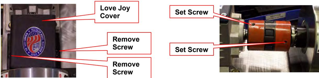
4. With someone holding up the end of the motor remove the four (4) bolts holding the motor / gearbox assembly to the mounting plate. Remove the complete motor, gearbox, cord & switch assembly from the machine. Save the mounting bolts to remount the motor / gearbox.
