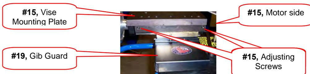
16. Once you are satisfied with the adjustments tighten the five gib mounting bolts and recheck your adjustments. This procedure may take a few tries. You can now remount the vise to the mounting plate.
