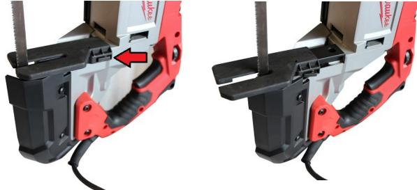
Push the button on the side of the blade guard (red arrow shown above) to extend the guard in the in the farthest outward position as shown in the 2<sup>nd</sup> picture above.
