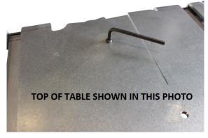
Install the 7/8" long set screw from the bottom of the table so the top of the fastener protrudes through the top of the table  $\sim 3/16$ ".
