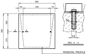
Position the machine on a firm cement floor, maintaining, at the rear, a minimum distance of 800 mm from the wall; anchor it to the ground as shown in the diagram, using screws and expansion plugs or tie rods sunk in cement, ensuring that it is sitting level.
