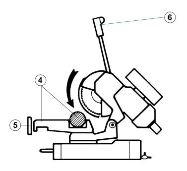
The cropper is now ready to start work, bearing in mind that the CUTTING SPEED and the TYPE of DISC - combined with a suitable descent of the head - are of decisive importance for cutting quality and for machine performance (for further details on this topic, see below in the chapter on "Material classification and choice of disks").
