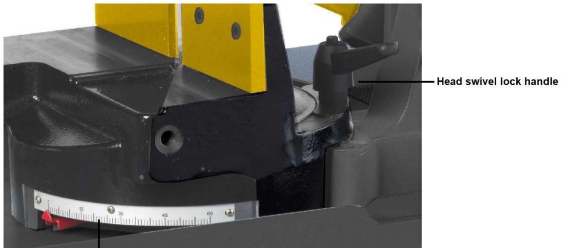
Miter scale. Preset stops at 0-45-60 degree angles.
