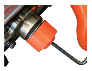
Begin tightening the bolt by holding with one hand the Allen wrench on the bolt, and holding with the other the block adapter/modeling block assembly flush against the starter tube. Some slippage may occur initially. Also, depending on the metal tube wall thickness, some pre-loading may be required on thin gages.
