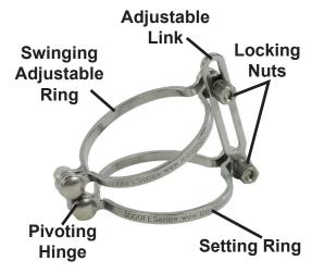
The patented **icengineworks**® tack-welding clamps have been specifically designed to simplify the actual fabrication of complex multi-section exhaust headers and other tubular projects that need to be welded, or even joined together like when using V-band clamps. When properly used these clamps will reduce, or even replace the need for complete assembly jigs and other traditional supporting devices giving the fabricator a new level of efficiency and flexibility.
