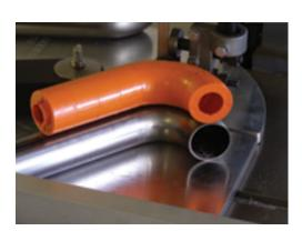
With the metal U-bend securely tight around the cutting spacer it's time to make the cut.
