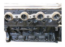
Plan ahead of time the key features in your intended design such as the OD and target lengths of the primary runners, based on experience or calculated. Decide if the runners will be equal-length, have steps, etc.; choose the type, number and location of the merge collectors.
