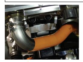
Having all the metal parts cut and ready to be tack welded, the actual fabrication for each exhaust header runner can start at either end of it. Separate the cut sections for each runner according to the Control Sheet created for this specific project.
