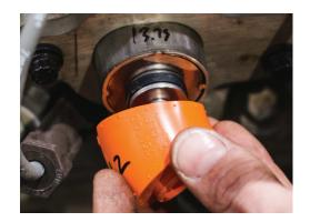
Next, insert the large-OD end into the starter tube while making sure that there are no gaps between the icengineworks® modeling block and the large-OD inner metal disk in the block adapter.
