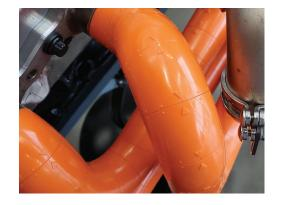
The icengineworks® modeling blocks have arrows molded at each end. When aligned, these markers indicate when those consecutive blocks can be sourced from the same J- or U-bend metal section during fabrication. Of course, this is true provided that they all have the same CLR.
