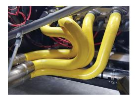
When you are satisfied with your exhaust header model and it feels right in every sense, take some additional time to carefully review each runner to make sure that there are no unwanted gaps or that the modeling blocks, specially those at the weld joints, have not moved or rotated unexpectedly. Misalignments or gaps will introduce errors and inaccuracies when the metal version is built. Make sure witness line alignments among blocks in constant-CLR curved sections remain 'zero-ed' in.
