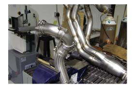
When all the joints have been tacked, loosen the nuts at the adjustable links icengineworks<sup>®</sup> tack welding clamps and carefully slide the clamps out of the runner.
