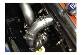
First, slide the setting ring of the icengineworks® clamp (the one with the fixed end on the adjustable link) about 1/8" from the end of the first tube to be joined (the first tube should be the one with the 'most straight' end of the two tubes to be joined). Spin the icengineworks® clamp until the swinging ring follows the curvature of the second tube end according to the design.
