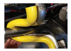
Based on the design you have in mind, it is easier to start it beginning with the cylinder that seems to pose the biggest challenge. By laying out the most difficult pathway first, the rest of the design will become progressively easier to figure out.
