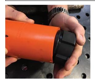
To get started, an intial icengineworks® plastic modeling block of your choice needs to be anchored to the open end tube coming from the exhaust header collectors, downpipe, catalytic converter, etc.
