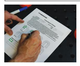
Fill out a U-Bend Metal Tubing Control Sheet for FESeries from the pad included following the printed directions. Each curved modeling block is 15-deg and it is represented in the U-bend drawings on the Control Sheets. Color as many empty blocks in the drawing as the number of blocks in each section in your design including the straight sections.
