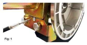
Fig: 1 shows the lower bolt for tensioner arm interfering with miter table mounting bracket .
