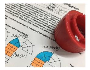
The process starts by designating pie sections in the drawings that correspond to each block section in the model. Each section in the drawing will require a label that identifies what cylinder it belongs to and its order within it (such as section 2C, meaning the third section in the runner for cylinder 2, etc.). Straight sections will have their own label.
