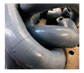
After setting up the first block in each runner using the neoprene block adapters, begin laying out blocks to start the design. In EQUAL LENGTH MODE sections will be created of known length (in inches) that will contribute to develop turbo manifold runners of precise lengths (measured at the imaginary centerline).
