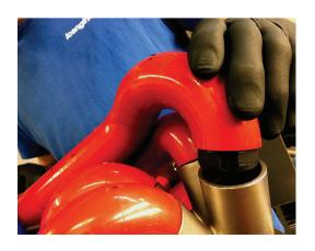
Any icengineworks® NPSeries modeling block can be anchored to an open pipe end of the manifold flange (starter pipe w/ round profile) or the turbocharger collector, to get the design started. Choose the design direction: following the gas flow direction (head to turbo), or going upstream (turbo to head) based on clearance, appearance, design complexity, welding sequence, etc.
