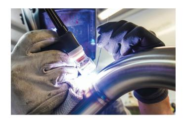
With all the curved and straight pipe sections cut per your Control Sheet, begin replacing them in your model. **Plan ahead the welding sequence to avoid dead ends.** Place at least 3 tacks around each joint that form the manifold runners for safety. Adjust accordingly until assembly is ready to be fully welded. Follow industry standard manifold welding procedures and techniques to complete your design.
