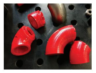
For the 1250NPSeries this requires the following blocks: For Short Radius elbows (SR, marked as 1-1/4"-CLR), use blocks labeled 45-deg/1" long to form multiples of 45-degree sections (45-deg, 90-deg, etc.). This particular block also measures a 1.000" arc length at the centerline so it is also used in EQUAL LENGTH MODE.
