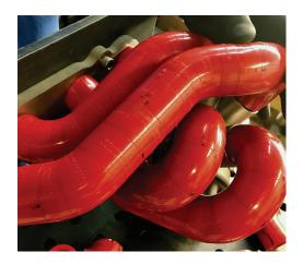
With little practice, it becomes evident how easy it is to design for the least amount of components or work required. Complex designs can always be revised to reach a simpler version to reproduce, for example in cases of hard-to-reach weld joints.
