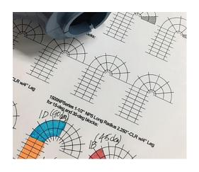
The process starts by designating pie sections in the drawings that correspond to each block section in the model. Properly label each section in the drawing identifying what cylinder it belongs to and its order in it to avoid confusion. For example: section 2C, meaning the third section in the flow direction in runner for cylinder 2. Straight sections will have their own label.
