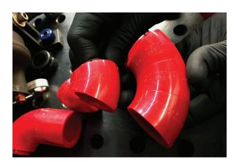
For the 1250NPSeries this requires the following blocks: For Short Radius elbows (SR, marked as 1-1/4"-CLR), use blocks labeled 45-deg/1" long **only** to form 1"-long or longer sections in 1" increments. For Long Radius elbows (LR, marked as 1-7/8"-CLR), use the 30-degree/1" long blocks **only** to form 1"-long or longer sections in 1" increments.
