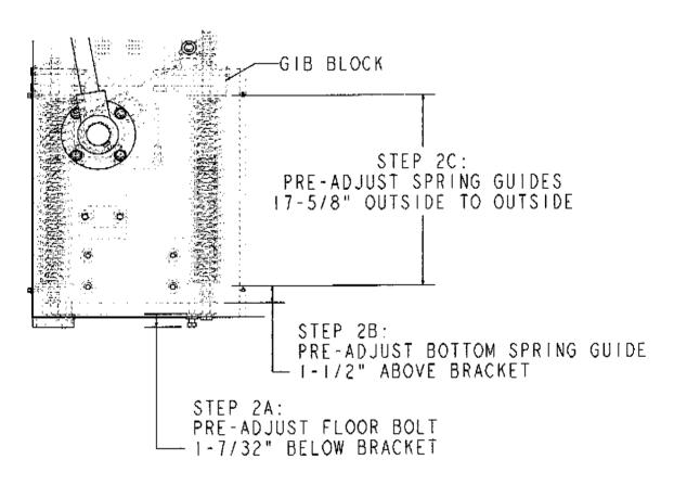
YOU CAN FINE TUNE THE SPRING ADJUSTMENT TO YOUR LIKEING BY RAISING OR LOWERING THE DIMENSION IN STEP 2C, BUT FIRST, GET ANY BINDS OUT OF THE MACHINE BY PERFORMING STEP I.
