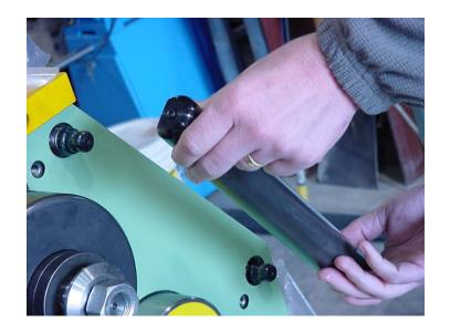
Remove cylindrical guide roll from machine after removing standard tooling from lower shafts (not shown)
