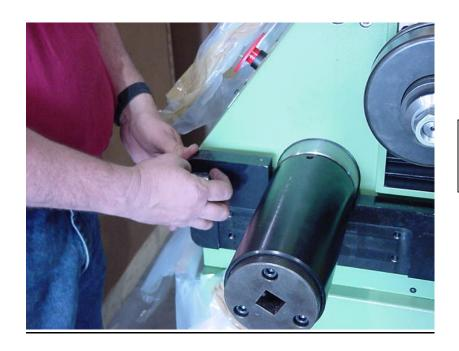
Secure mounting plate with nuts
