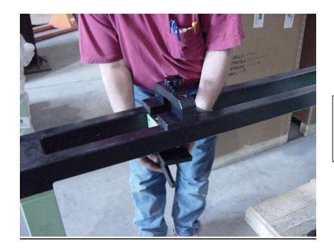
Install the slide block to the rails and secure into position with threaded handle
