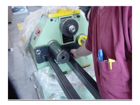
Secure rail to plate with bolts
