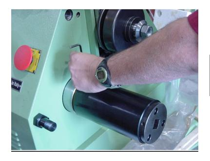
Install collar sleeve on lower shaft and tighten set screw
