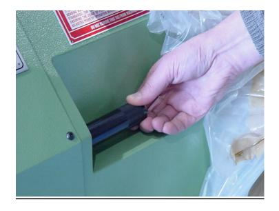
Remove guide roll adjusting screw
