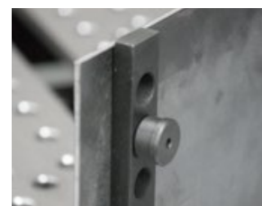
Magnet keeps sheet metal in vertical position
