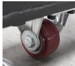
Two casters for quick repositioning of manipulator.
