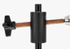
Reinstall spindle and pad in opposite direction pointing up.
