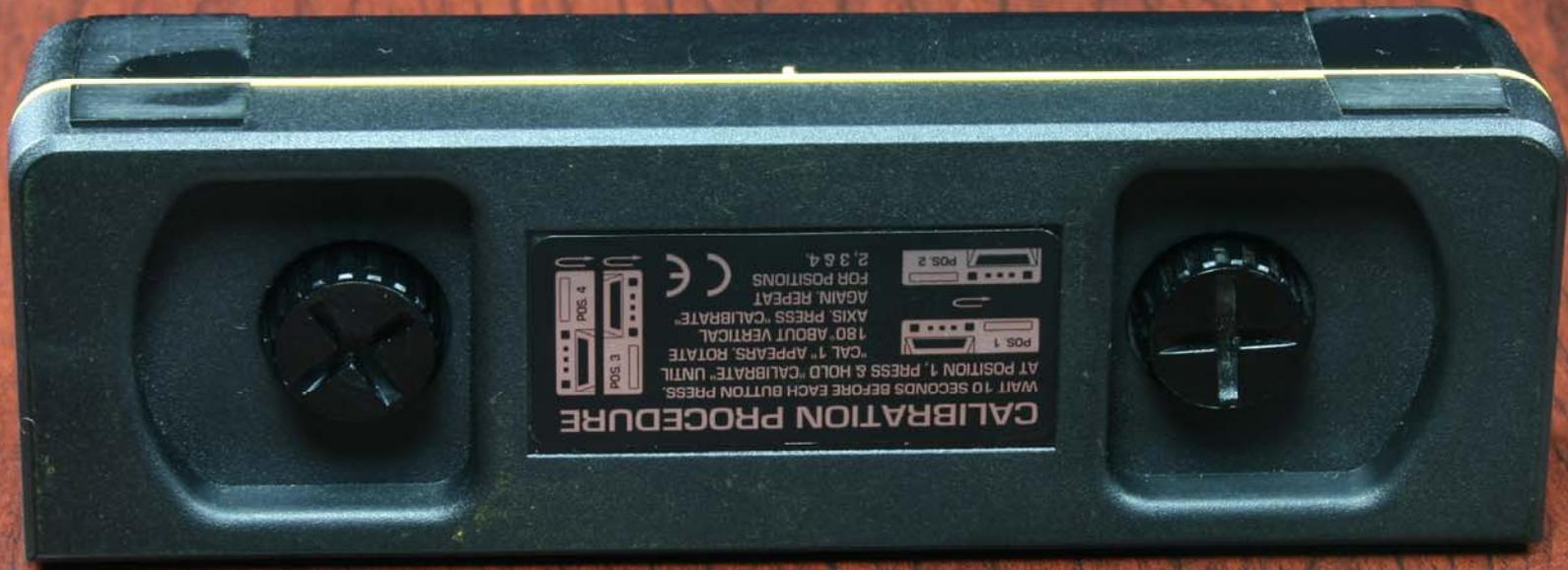
Turn the SmartTool end for end so it is facing away from you, still with the LCD display down. After display stops changing, carefully press and hold the “Calibrate” button until “Cal 2” shows on the display. (See picture inset)
