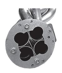
The top and middle plates separated by spacers serve as solid guides to create incoming tube runner designs that are parallel on their last inch of length for an easy header assembly and fabrication, and streamlined exhaust flow.
