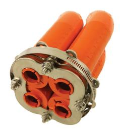
The icengineworks® Collector Dummies can be secured to the chassis, frame or other temporary support utilizing angle or flats to create a simple non-intrusive structure that can be clamped on, spot welded or bolted down using the extended flats and/or holes (1/4-inch bolt size) provided on the CD top plate.
