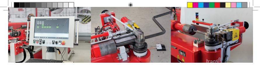
The DB 2060 3A-CNC-R mandrel bending machine performs tight radius bends with the highest quality. The machine meets all industry standards and exceeds customer expectations. This machine was designed specifically for bending handrails.
