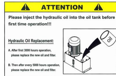
Figure 12. Fill with oil before use.
