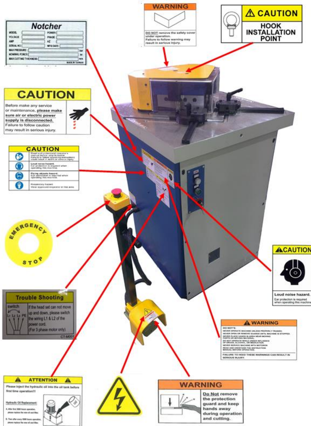
Figure 11. Hook installation point
