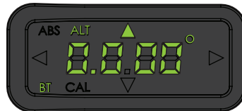
Figure 5. Device display in Alternate zero mode
