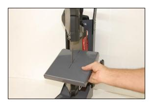
3. Insert the shoe into the slot, located on the under-side of the EZ-SLIDE-IN TABLE.
