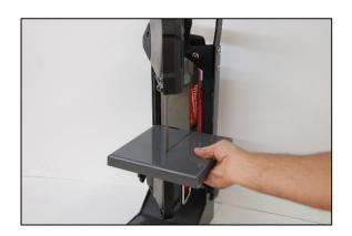
5. Clamp the EZ-SLIDE-IN TABLE in place, by twisting the knob clockwise.
