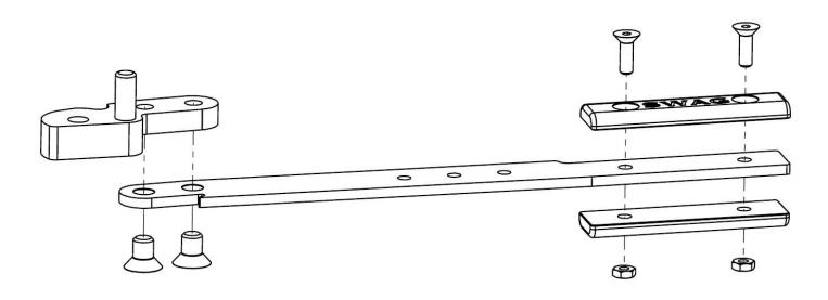
Step 3: Attach the Arm (4) to the Pivot (3) using the two 1/2"-13 x 3/4" (7) as shown above. Then attach the Upper and Lower Grip (6 & 20) to the arm using the two 5/16"-18 x 1" (18) and the 5/16"-18 Thin Jam Nut
