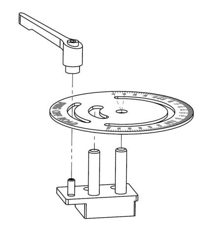
Step 1: Attach the Degree Wheel (8) to the Base (1) as shown above. The easiest way to attach the Handle (14) to the threaded PEM Stud (17) is to pull up against the spring pressure in the handle and use an Allen key to tighten the bolt down. This will allow the handle to stay stationary while the internal barrel threads onto the stud.
