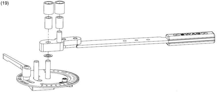
Step 4: Drop the 1/2" x 7/8" Washer (11) onto the pin that is in the middle of the Degree Wheel and then slide the arm assembly onto the same pin as shown above. The optional bend radius tubes (9 & 10) can then be added to the center pin and the pin that is press fit into the pivot.
