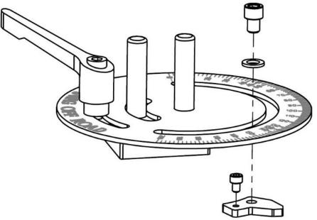
Step 2: Attach the Bend Stop (12) to the Degree Wheel using the provided 10-24x1/4" (13) and the 5/16"-18 x 3/8" (16) with the 5/16" Washer (15) on the larger bolt. Orient the stop so the pointer sticks out from under the degree wheel and the rectangular protrusion points towards the Handle as shown above.
