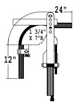
(IMPORTANT) WITH YOUR TUBE BENT TO 90°, BUT STILL IN THE BENDER, CHECK TO SEE IF THE EDGE OF YOUR DIE IS STILL LINED UP WITH YOUR MARK. IF IT IS, YOU'RE O.K. IF NOT, IT WILL BE NECESSARY TO CUT ANOTHER PIECE OF TUBING AND REPEAT THE TEST. THE MARK MUST BE LINED UP WITH THE DIE IN ORDER TO GET ACCURATE INFORMATION.
