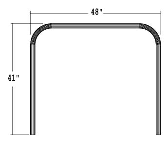
WE NOW HAVE OUR ROLLBAR COMPLETED AND IT MEASURES 48" WIDE AND 41" HIGH. REMEMBER, EXTRA TUBING WAS FIGURED IN ON OUR DOWN LEGS ON PURPOSE AS A SAFETY FACTOR AND BECAUSE IT IS EASIER TO CUT A LITTLE OFF THAN TO HAVE TO ADD SOME ON.
