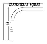
IT WILL BE NECESSARY TO CHECK YOUR BEND WITH A CARPENTER'S SQUARE TO VERIFY THAT YOUR 90° BEND IS ACCURATE.
