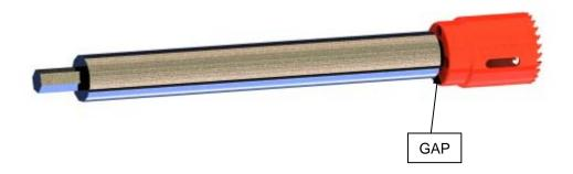
TO SOLVE THIS PROBLEM YOU WILL NEED TO USE A SIMPLE WASHER. PLACE THE WASHER BEHIND THE HOLD SAW AND TIGHTEN. THE WASHER SHOULD BE THICK ENOUGH TO TAKE UP THE GAP.
