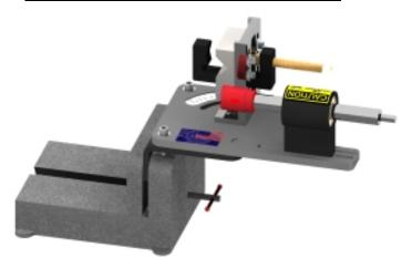
IF YOU ARE GOING TO USE THE NOTCHER IN A HORIZONTAL POSITION, IT WILL BE MECESSARY TO FABRICATE A STAND THAT WILL SUPPORT THE UNIT PROPERLY. CLAMPING THE UNIT IN A VISE, WITHOUT PROPER SUPPORT, WILL CAUSE THE NOTCHER TO FLEX AND CUT OFF CENTER.
