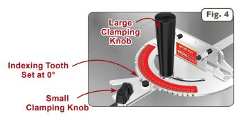
2 Loosen the (4) Phillips head screws that secure the faceplate to the protractor, and depending on your application, square the faceplate to the blade, miter slot, sanding belt, etc. **NOTE:** When squaring to a saw blade (see **Figure 5**), use a reliable square for this important alignment. Securely retighten the (4) Phillips head screws to complete the alignment.
