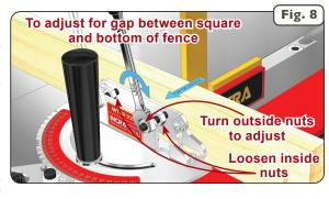
the bracket as shown in **Figure 8**, and then tighten the other outside nut by the same amount in the same direction against the rear leg. Alternate this 1/6 turn procedure between the two nuts until the fence is perfectly square to the table DO NOT TURN THE SET SCREW and DO NOT over tighten the nuts. It usually takes less than 1 full turn of the nuts to square your fence to the table.
