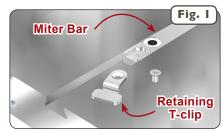
2 Using the supplied 3/32" hex key, adjust each of the (3) visible miter bar expansion disks for a zero-side play, sliding fit in your miter channel as shown in **Figure 2**. Turning the fastener clockwise EXPANDS the bar width. The disks are designed to require a fair amount of adjustment torque for proper expansion.
