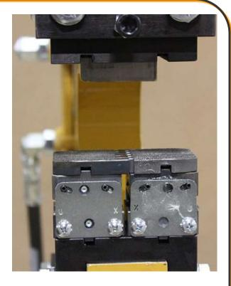
In this view it will shows how to remove the jaw caps. Insert a screw driver into the machined slot to break the magnetic force.
