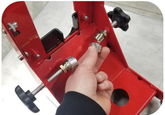
7. With the top arm standing in the upright position, install the portaband saw in the jig, roughly centered in the cutout in the top arm. Be sure that the front handle is installed as far forward in the arm as possible.
