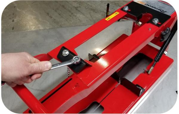
**2.** Using a 1/2" wrench, remove the two 5/16" bolts from the front handle bracket.
