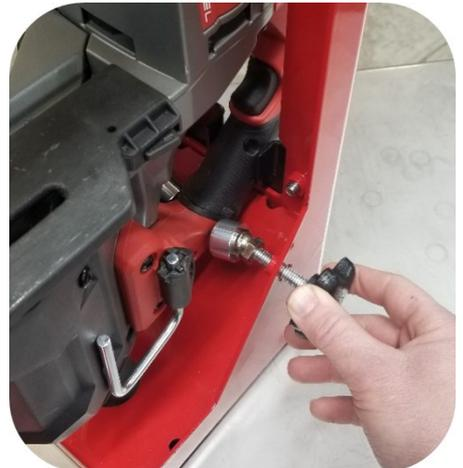
9. Pivot the base of the jig up to meet the bandsaw. Check blade alignment within the slot in the base. Using a 3/4" wrench, slightly loosen the three bolts at the base of the jig so that it can be adjusted for blade alignment.
