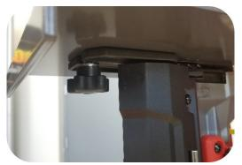
3. Slide the table over the material guide and into the small slot at the back of the saw. Clamp the washer and hand knob to the bottom of the guide.
