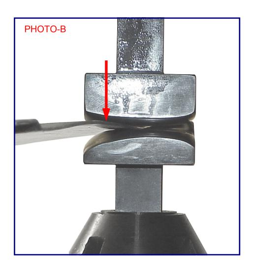
**STEP D.** You are ready to shrink, at this point. Start machine on low speed. Push metal in and pull back out using the same path. As the metal is pushed in, a pucker is pulled in the metal. As you pull the metal out, the pucker is flattened. If the dies are set properly, the metal will show signs of shrinking. It will also have some waves, as in the photograph. Try to keep it as smooth as possible. The panel will need to be planished for final smoothing. (SEE PHOTO-C)
