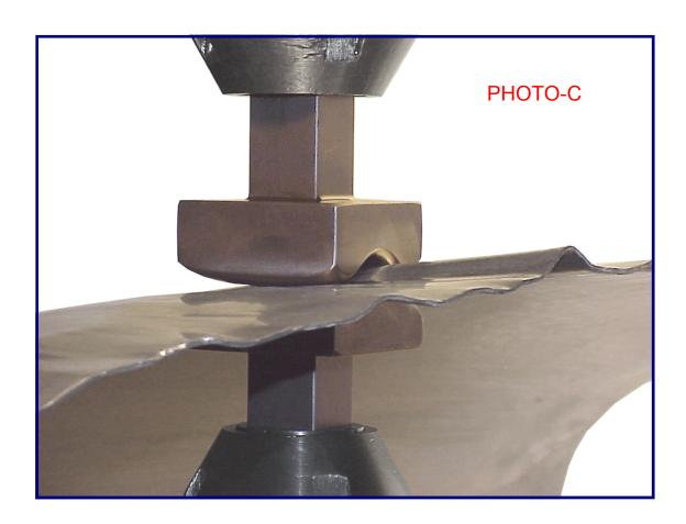
**STEP E.** When shrinking a panel, you have to run more passes on the outside than you do on the inside. #1 will require fewer shrinks than #2 and #2 will require less than #3. The number will depend on the severity of the amount to be shrunk. (SEE PHOTO-D)
