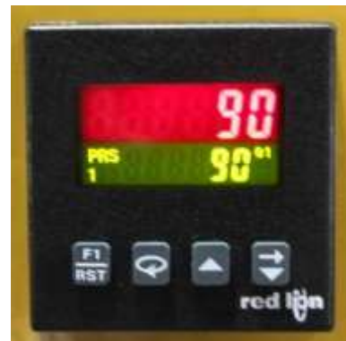
Stop position with 90° Preset Stop Point.
