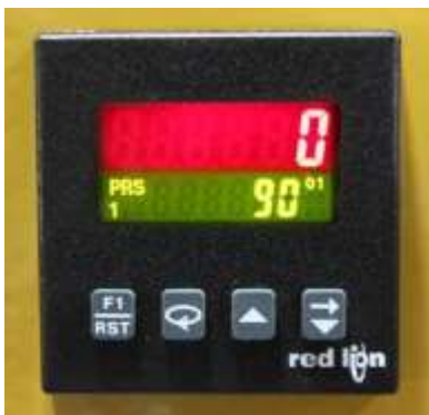
Home position with 90° Preset Stop Point.
