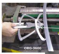
The ORG-3600 folds for easy storage. To unfold, loosen white thumb nuts, swing each arm to its limit, then re-tighten.
