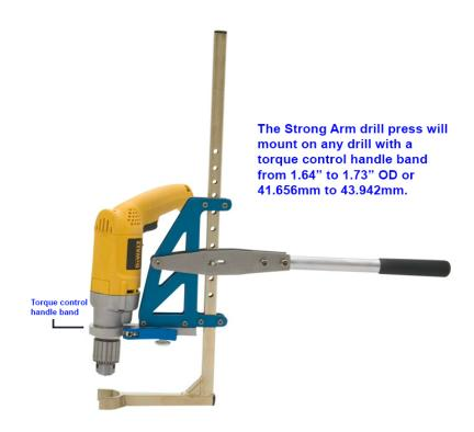
The Strong Arm 5 portable drill press fits most electric drills that have a clamp on anti-torque handle. The Strong Arm 5 will mount on the drills torque control handle band if it is from 1.64" to 1.73" OD. The two drill brands with a consistent dimension that work with the Strong Arm 5 drill clamp best are DeWalt and Ridgid but many others are possible. If you are using a drill that has a larger band, or a cordless or pneumatic drill, then you will need an optional Drill Chuck Adapter.
