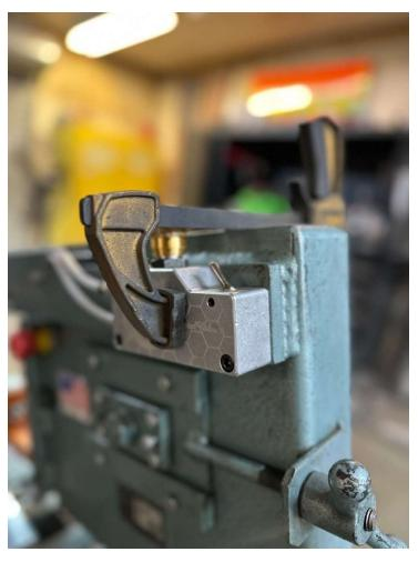
2. Clamp your new SpeedValve body to the .75"x2" solid bar welded into the top of your bow. Exactly where is entirely up to you. However, I like at the front of this bar. Using a transfer punch, mark your mounting hole locations into the .75"x2" bar. Remove your clamp and valve. Use a #16 or 3/16 drill bit and drill all the way through, be sure not to hit your wheel and blade on the other side. Now tap the holes for 12-24 threads.
