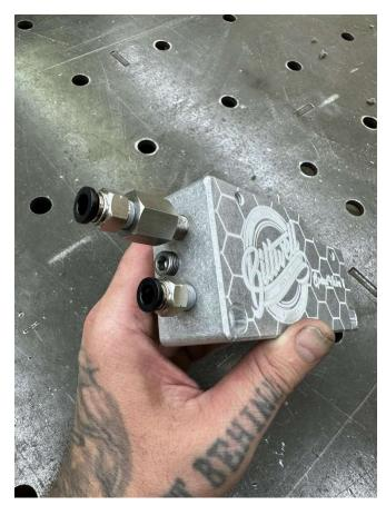
5. Route the provided oil lines through the cable chase covering your OEM power cord (this may require notching the end tab and/or trimming the length down depending on saw model). Connect the bottom fitting of your cylinder to the straight push connect fitting at the back of the Speed Valve. Trim to fit. Now connect the top fitting in your cylinder to the 90° fitting at the bottom of the Speed Valve below the toggle. Trim to fit.
