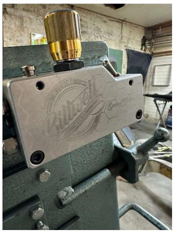
4. Install the provided 1/8 NPT plug into the center rear hole. Install the snubber into the top rear hole and install one of the provided straight push to connect fitting into the snubber. Then install the last provided straight push to connect fitting into the bottom rear hole. Install all of these using a thread sealant. I prefer LOCTITE 545 but Teflon tape will work as well.
