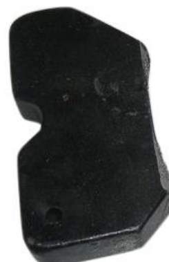
CAST ARBOR PLATES THAT FAILED UNDER LOAD
