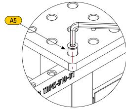
**NOTE**: After aligning the two Rhino Carts, check the level and adjust the leveling pads. This will ensure the Beams and Plate are flat when installed in the following steps.
