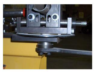
3. Select the material and insert it into the vise. Leave the minimum required material hanging beyond the vise.
