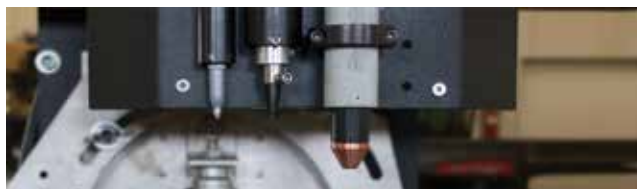
Tool changer: Machine will switch between marker/etcher/plasma/laser pointer automatically depending on your intended tasks.
