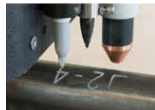
Tube marking/etching: Bend-Tech Dragon obtains the bending information from the Bend-Tech Industrial software to automatically mark and etch bend angle labels, bend locations and rotations.
