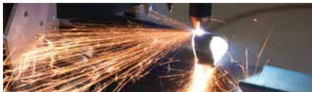
Plasma cutting: Cuts end profiles, holes, and other contours.
