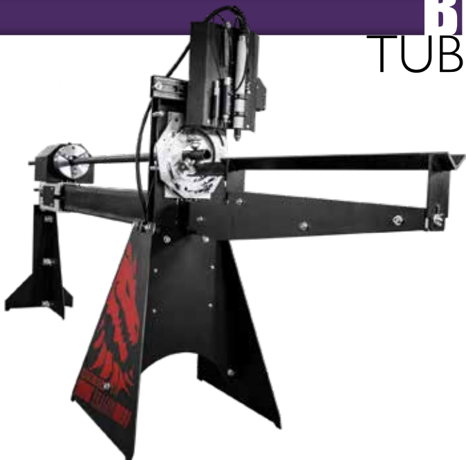
Plasma cutting: Cuts end profiles, holes, and other contours.
