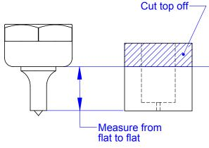
Coupling Nut 2200-504 Cut urethane stripper to match
